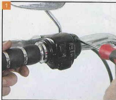
1 Use a T25 Torx driver to remove one of the bolts in the clutch perch clamp.
