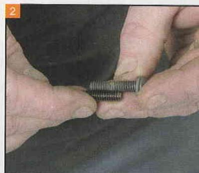
2 The RAM Mounts Kit comes with a variety of bolts for different applications. Compare the threads of the stock bolt to the bolts included in the kit to choose the correct ones for your application.
