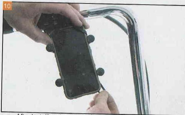
10 After installing the phone in the X-Grip®, further secure the phone on the corners with the rubber tether.
