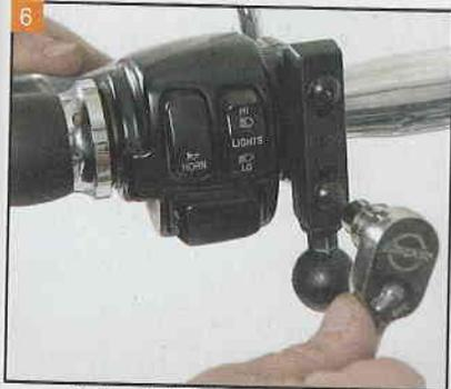
6 Uniformly tighten the mounting bracket with an Allen wrench.
