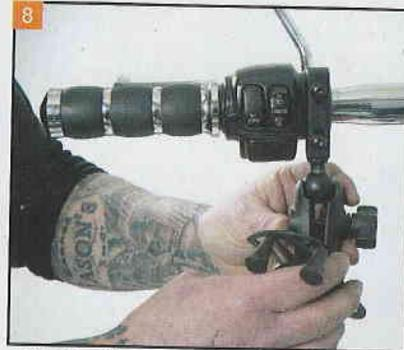
8 We used the separate, shorter, double-socket arm for this application, compared to the longer arm included in the kit.
