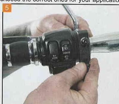
5 Install the mounting bracket with hardware. Start the bolts by hand into the threaded holes of the clutch perch. Because of the height of these handlebars, we position the ball mount down. It can be installed either way.
