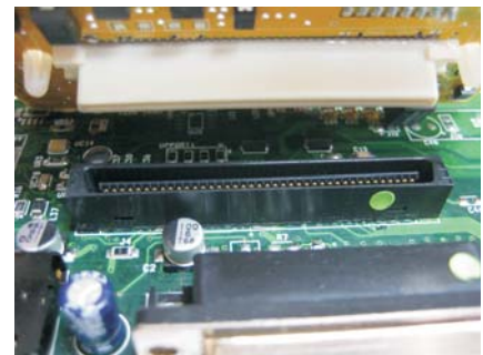
Internal view of ribbon connector and Port Replicator 1
