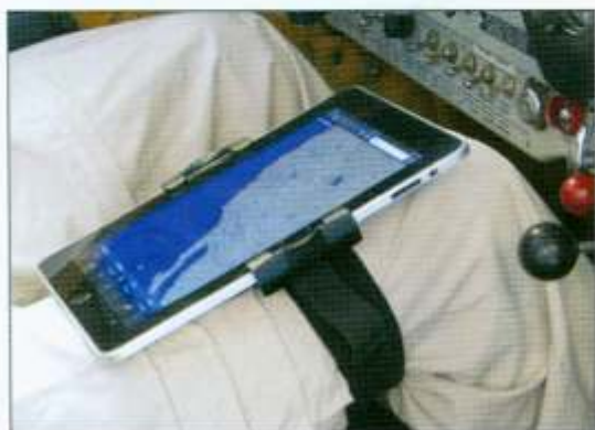
MyClip Thing, left, clamps the iPad with an elastic strap and two soft clips.
